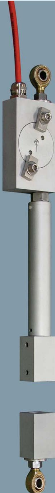
The RST Tunnel Profile Monitoring System is a series of linked rods, fixed to the tunnel wall, to monitor deformation. A data logging system and related software is available to provide near real time displacement and generate a graphical representation of tunnel performance.
