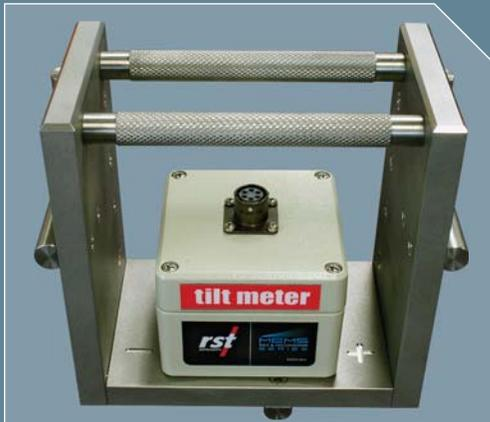
RST Portable MEMS Tilt Meter
