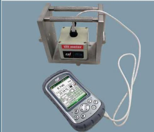
Digital Portable Tilt Meter with Field PC Readout
