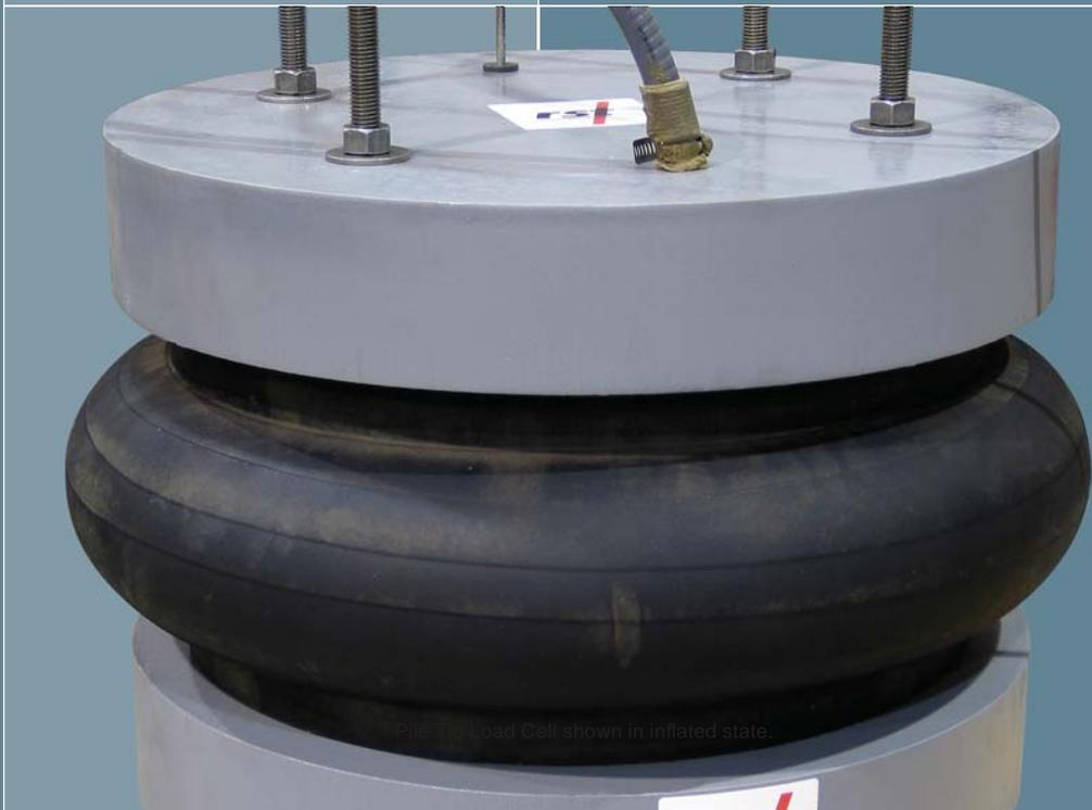
Pile Tip Load Cell shown in inflated state.
