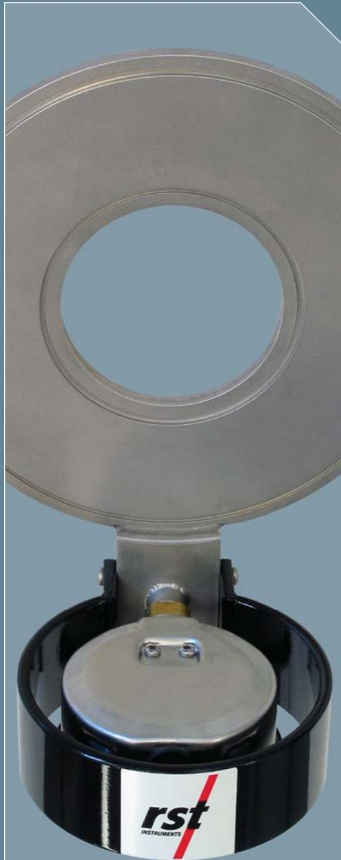
Hydraulic Load Cells are constructed from stainless steel. The load is distributed equally over the loading area of the cell by a thick, machined steel distribution plate. The load, when applied to the cell, causes a pressure increase in the hydraulic fluid, and this change in pressure may be measured via a Bourdon Tube Gauge or a variety of electrical transducers.
