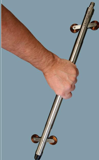
The RST Digital MEMS Inclinometer Spiral Sensor is used to determine down-hole helical deformation of installed inclinometer casing. Installed casing spiral is a function of the manufacturing process, casing coupling, and installation technique.
