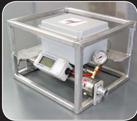
Solution Grout Monitor Unit
