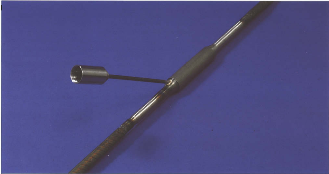
P-300 reinforcement strain gauge welded to steel bars
